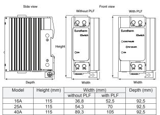
**WARNING**: To reach the thermal performance the gap between two ESwitch power contactors must be at minimum 10mm.
